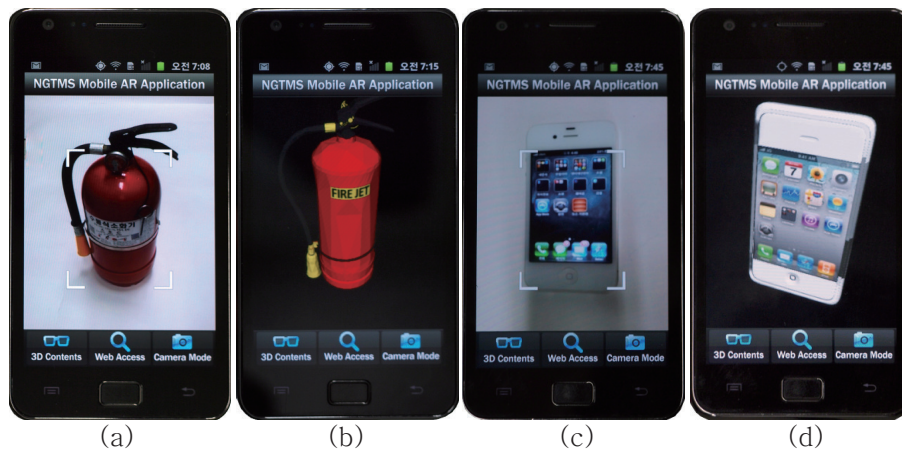
Figure 9: Experimental results using a SHW-M250S in front of a clean background: (a) Object recognition of a fire extinguisher through the phone camera, (b) Corresponding 3D contents display of (a), (c) Object recognition of an iPhone through the phone camera, (d) Corresponding 3D contents display of (c)
